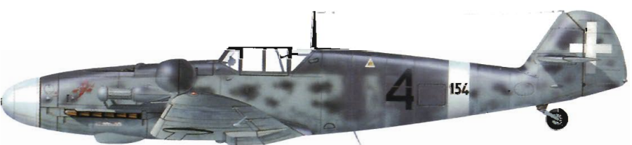
▲ Messerschmitt Bf 109G-6/Trop 3° Gruppo CT, Regia Aeronautica The G-6 variant of the Bf 109 introduced more powerful 13mm (0.5in) guns over the engine. The swelling needed to fit the larger breeches gave the type its nickname of 'Die Beule', or 'The Budge'.
