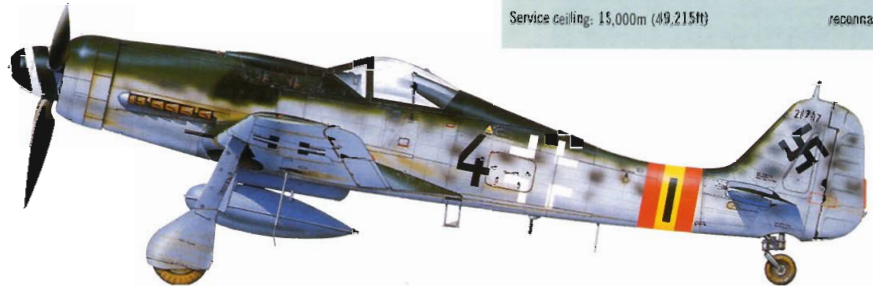
▲ Focke-Wulf Ta 152H-1 Jagdgeschwader 301 The 'H' variant of the Focke-Wulf Ta 152 was a high-altitude fighter. Small numbers were operated by JG 301, primarily to provide cover over Me 262 bases while the jets were taking off and landing.
