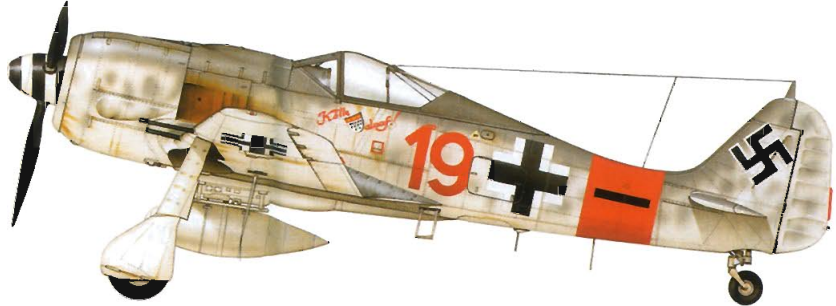
▲ Focke-Wulf Fw 190A-8 5. Staffel, JG 300 The A-8 was one of the major production variants of the Fw 190. Known as the 'Panzerbock', it carried four 20mm (0.8in) cannon in the wings and a pair of MGs over the engine. This example was flown by Unteroffizier Ernst Schroeder.
