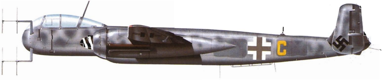
Specifications Crew: 2 Powerplant: 2 x 1342kW (1800hp) DB 603 Maximum speed: 585km/hr (363mph) Range: 1850km (1150 miles) Service ceiling: 9800m (32,150ft) Dimensions: span 18.5m (60ft 8in); length 16.34m (53ft 7in); height 4.1m (13ft 5in) Weight: 15,100kg (33,289lb) loaded Armament: 6 x 20mm (0.8in) MG 151/20 firing forward; 2 x 30mm (1.2in) cannon firing obliquely upward
