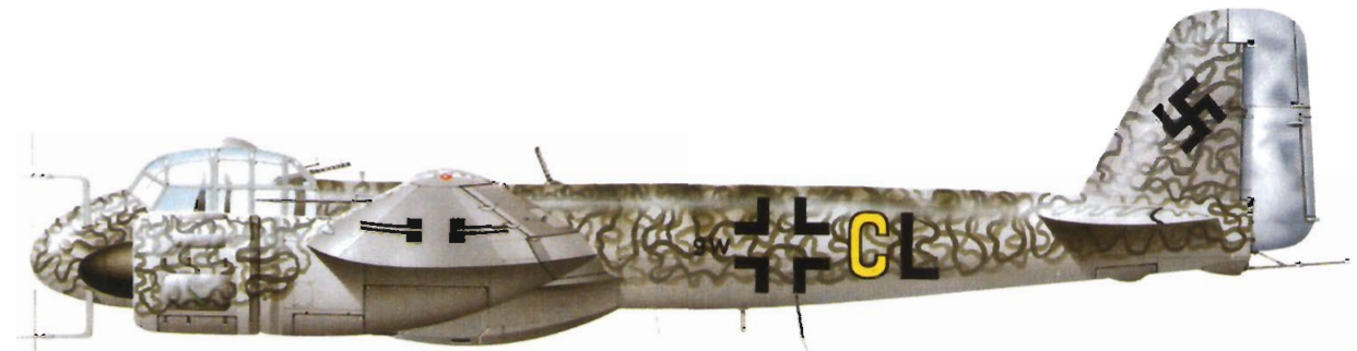
▲ Junkers Ju 88G-6b 1 Gruppe, Nachtjagdgeschwader 101 Based at Ingolstadt late in 1944, this Ju 88 carries the latest Lichtenstein SN-2 radar array and is armed with a pair of upward-firing MG 151 cannon in the centre of the fuselage.
