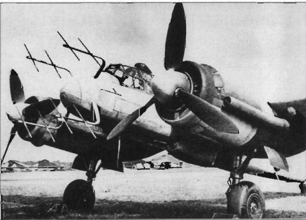
▲ Stag's antlers In the later version nightfighter variants, such as this Ju 88G-7A, the antennas were canted to reduce interference.
