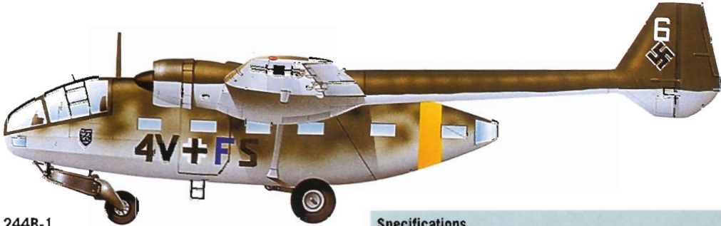
▲ Gotha Go 244B-1 4. Staffel, Kampfgeschwader zur besonderen Verwendung 106 Developed as a powered version of the Go 242 glider, the Go 244 was a potentially practical tactical transport which could never overcome its one fatal flaw: it was decidedly underpowered.
